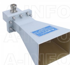
LB-284-10-C-7/16F Standard Gain Horn Antenna 2.6-3.95GHz 10dB Gain 7/16(DIN) Female
